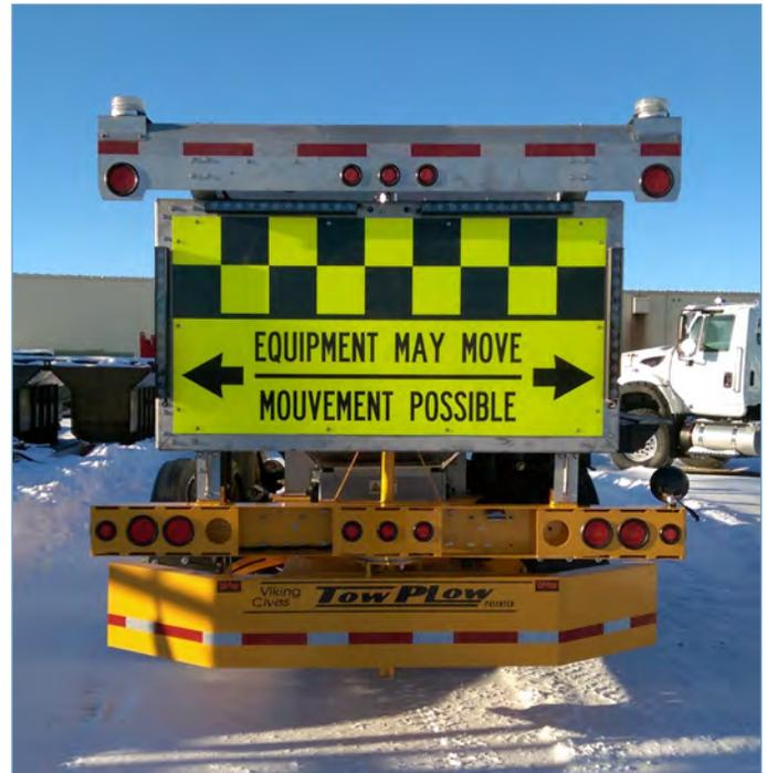
New sign on the back of a tow plow.
